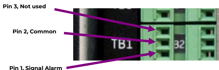
Figure 37 Alarm Output Wiring
