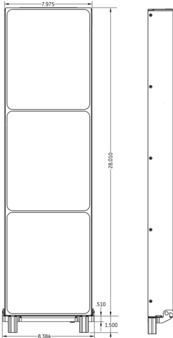
Note: Cold plate quick disconnects not shown. Liquid connection fitted with SAE -4 thread (7/16-20) coupling.
