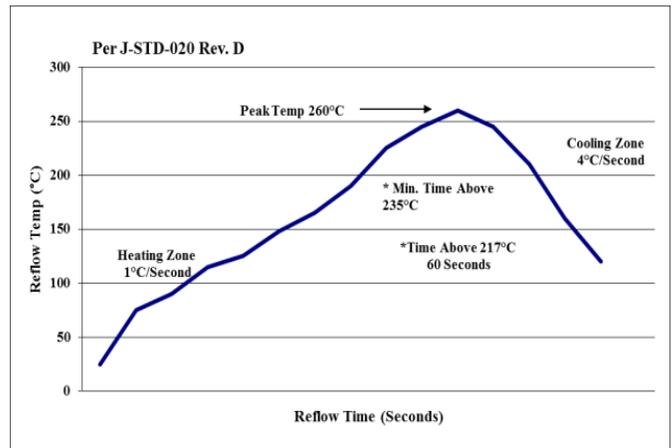
Figure 23. Recommended linear reflow profile using Sn/Ag/Cu solder.
