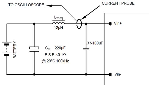
**Figure 7. Input Reflected Ripple Current Test Setup.**
