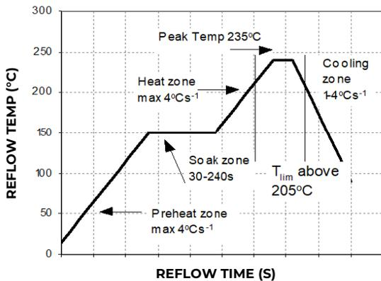
Figure 21. Reflow Profile for Tin/Lead (Sn/Pb) process.
