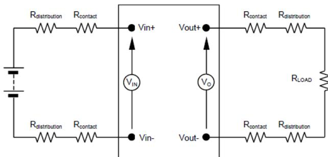
**Figure 9. Output Voltage and Efficiency Test Setup.**
