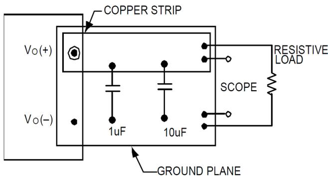
**Figure 8. Output Ripple and Noise Test Setup.**
