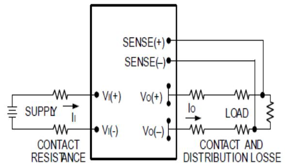
Figure 11. Circuit Configuration for remote sense .
