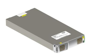
The OmniOn IR025H3R240ATEZ true three-phase rectifier efficiently transforms energy from any standard three-phase source into 240 volt DC power needed for industrial applications. The rectifier operates using three-phase input voltages from 320 to 530 VAC without the need of a neutral conductor. This means that one single rectifier can be used globally to meet all your 240V powering needs.
