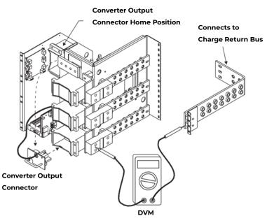
Figure 6-1: Voltage Measurement Points
