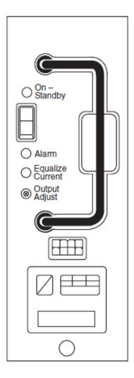
Figure 3-1: Front Panel of ES671 Converter
