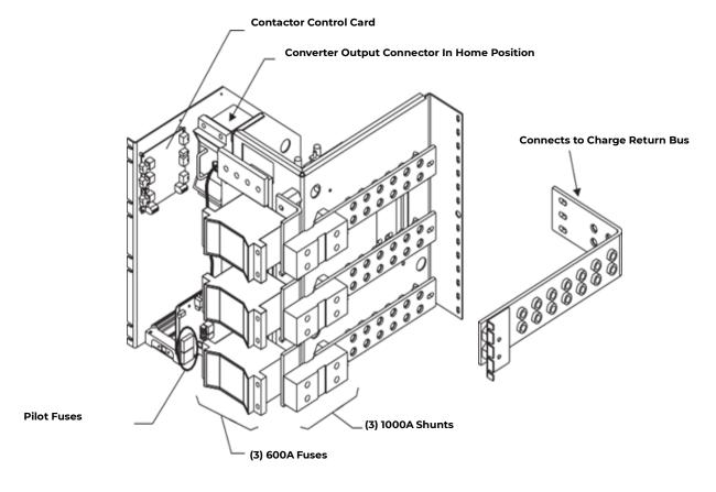
Figure 2-1: ED83143-30 Off Line Equalization (OLE) Panel
