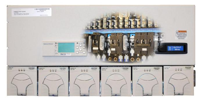
The shelf is installed with a minimum gap of 3/4 inch below the system to allow proper airflow. Attach the CPS shelf to the frame using a minimum of twelve (six on each side) of the 12-24 screws included with the shelf.
