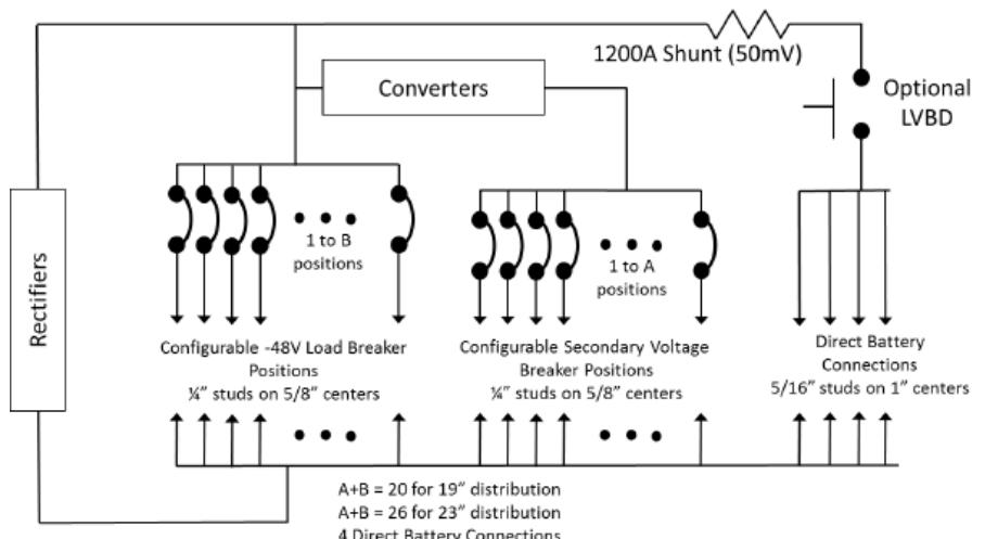
**Note:** (+) Battery Cable Connects to the Power System Return Bus!
